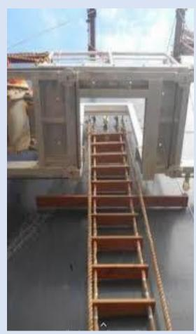
Several vessels with noncompliance trapdoor arrangement overcome this issue by using their accommodation ladder. Pilot ladder compination arrangement with an accommodation ladder rigged is acceptable if the below four conditions apply
