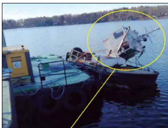
Tug wheelhouse torn from attachments.
